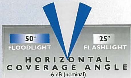
Floodlight delivers a 50° horizontal coverage pattern.
